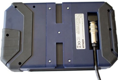
Fig. 10: Camera cable fed through guide
