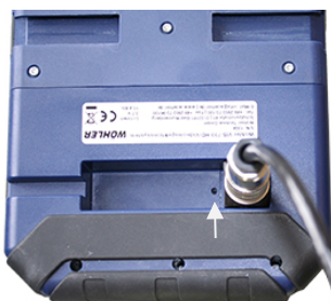
Fig. 56: Reset hole indicated by an arrow
