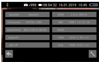
Fig. 41: Info menu with SOM (Firmware of the camera) and CAM (Version of the camera head)
