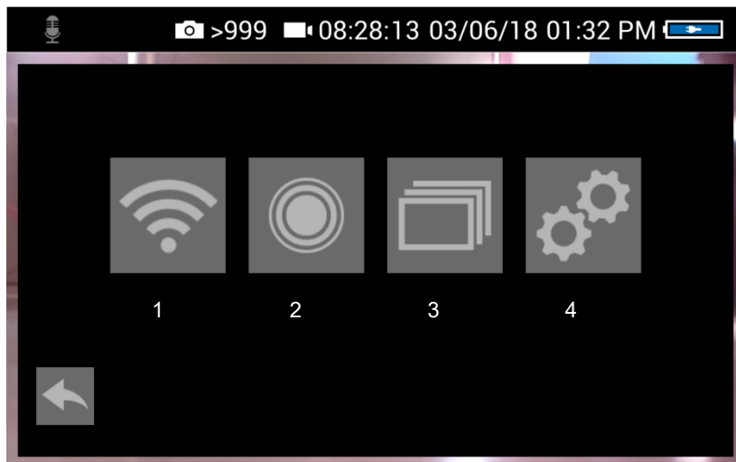
Fig. 28: System menu with submenus WLAN (1), Locator detection (2), Image and video gallery (3) and settings (4)
