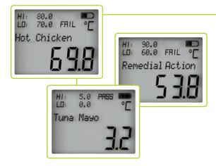
With the checklist items loaded onto the handheld, readings are stored with location, user, date, time and limits. Up to 1000 readings are stored before upload is required. Attach the appropriate type K thermocouple probe and store readings with the press of a button. Scroll quickly through your checklist with the ▲▼ buttons.
