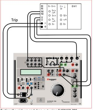
Testing the pick-up and drop-out using SVERKER 780
