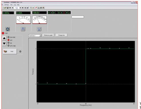
Testing frequency relay with SVERKER 780
