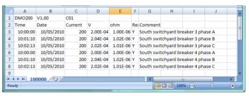
The DM0600 comes with the option of applying upper and lower pass limits for resistance and length of test for production line applications.
